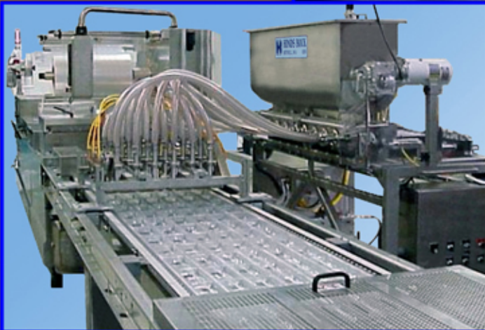
Fillers seamlessly integrate with horizontal vacuum formers and tray/cup/bowl sealers.
