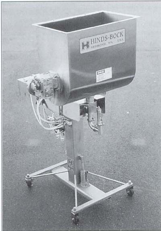
"U"-hopper with helical blade agitator
